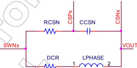
The individual phase current is summed into to the PWM comparator feedback in this way current is balanced is via a current mode control approach.
